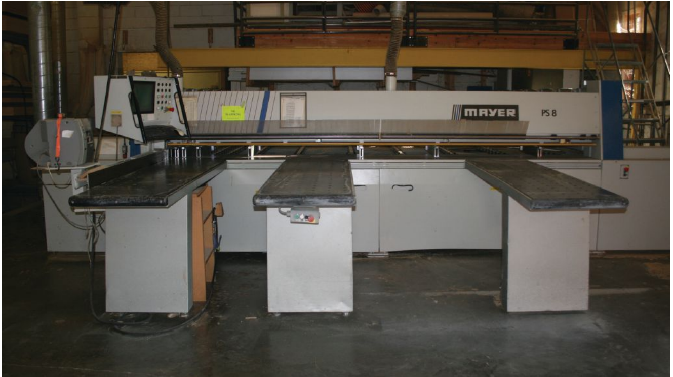
A Mayer panel saw, Busetto CNC machine, and a powder-coating alley (below) are among key production points for Greenberg Casework in all its market segments.
